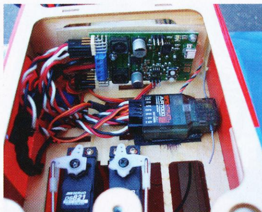
The SFX6 sound module circuit board nestles in nicely beside the Spektrum AR7000 receiver.
