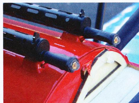
Details of the LED installation at gun tips. Note heat shrink holding them in place and covering wires.
