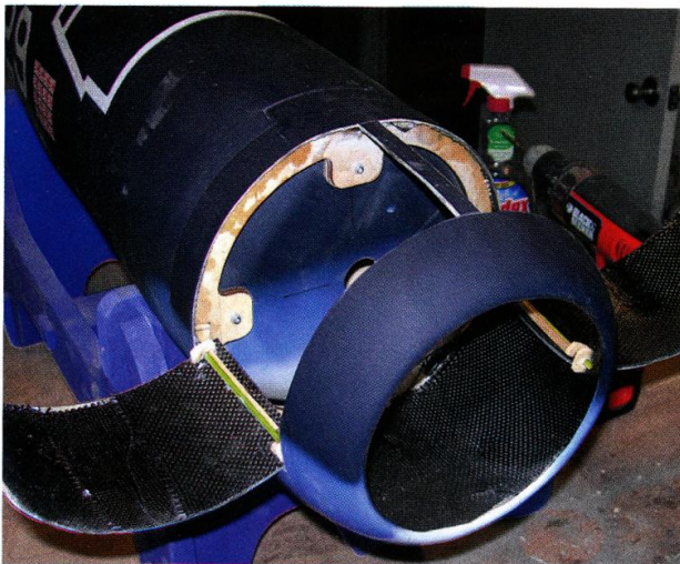
The side panels are then hinged back into place. This gives a quick way to replace the battery pack.
