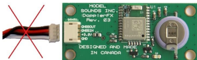
Figure 3 - Incorrect Position of 4-Wire Connector
