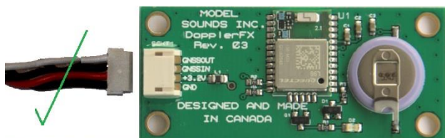
Figure 2 - Correct Position of 4-Wire Connector
