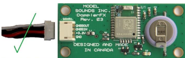
Figure 2 - Correct Position of 4-Wire Connector
