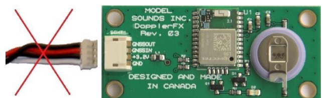
Figure 3 - Incorrect Position of 4-Wire Connector
