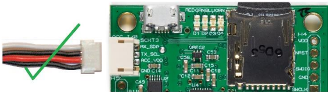
Correct Orientation of 4-Wire Connector
