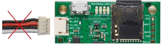
Incorrect Orientation of 4-Wire Connector
